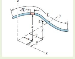
(2) Areas. When a body of density \_ has a small but constant thickness t, we can model it as a surface area A, Fig.  $^{\circ/\vee}$ . The mass of an element becomes dm = t dA. Again, if p and t are constant over the entire area, the coordinates of the center of mass of the body also become the coordinates of the centroid C of the surface area, and from Eqs. ( $^{\xi-\gamma}$ ) the coordinates may be written as
